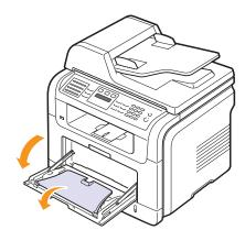
If you are using paper, flex or fan the edge of the paper stack to separate the pages before loading.
